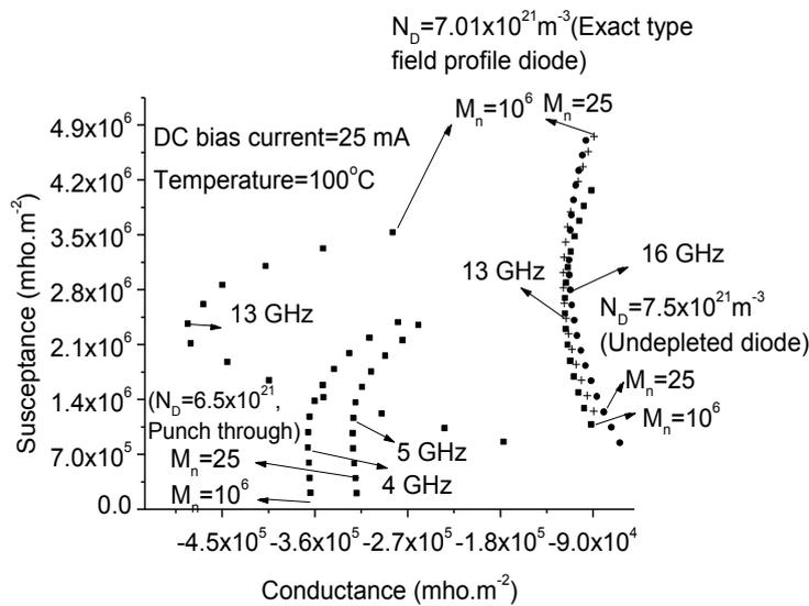
**Figure 2** Admittance characteristics of  $n^{++}np^{++}$  Si flat structure X band IMPATT diodes under different doping levels and multiplication factors.
