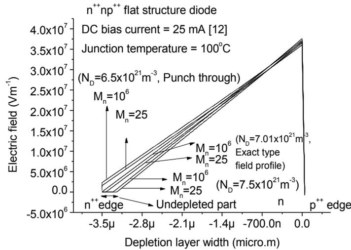
**Figure 1** Electric field distributions in the depletion layer of  $n^{++}np^{++}$  flat structure X band IMPATT diodes under different doping levels and multiplication factors.
